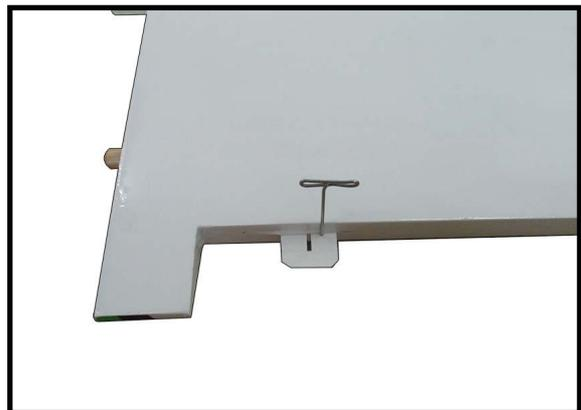
Slide the wing panel on the aileron until there is only a slight gap. The hinge is now centered on the wing panel and aileron. Remove the T-pins and snug the aileron against the wing panel. A gap of 1/64" or less should be maintained between the wing panel and aileron.
