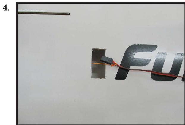
Attach servo lead to the aileron servo. Attach the string to the servo lead and carefully thread it though the wing. Once you have thread the lead throught the wing, remove the string so it can use for the other servo lead.
