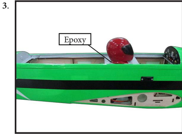
Position the canopy onto the fuselage. Trace around the canopy and onto the fuselage using a felt-tipped pen. Carefully cut and remove covering material from the fuselage where the canopy makes contact, exposing the bare wood. Then permanently glue the canopy in place with epoxy glue or special "canopy glue".
