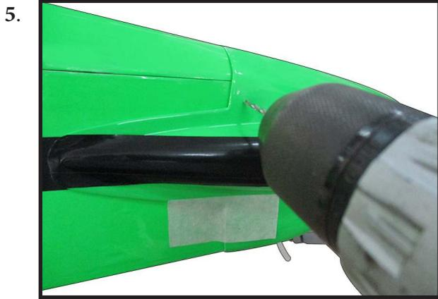
Install the muffler and muffler extension onto the engine and make the cutout in the cowl for muffler clearance. Connect the fuel and pressure lines to the carburetor, muffler and fuel filler valve. Secure the cowl to fuselage using the M3x10mm socket head screws. Putting a small length of silicon fuel tube under the head of the screw helps with vibration.
