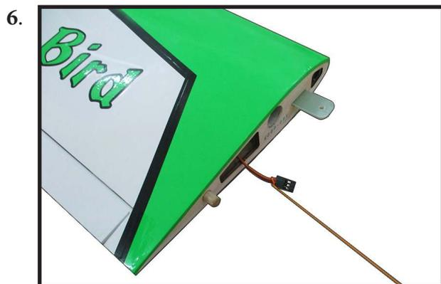
Tape the servo lead to the wing to prevent it from falling back into the wing.
