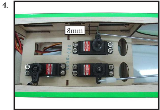
**RUDDER PUSHROD INSTALLATION**
