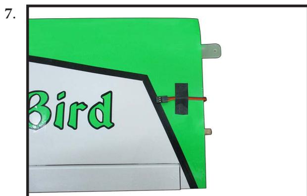
Reinstall the servo into the servo mount and secure the servo in place using the wood screws provided with your radio system.
