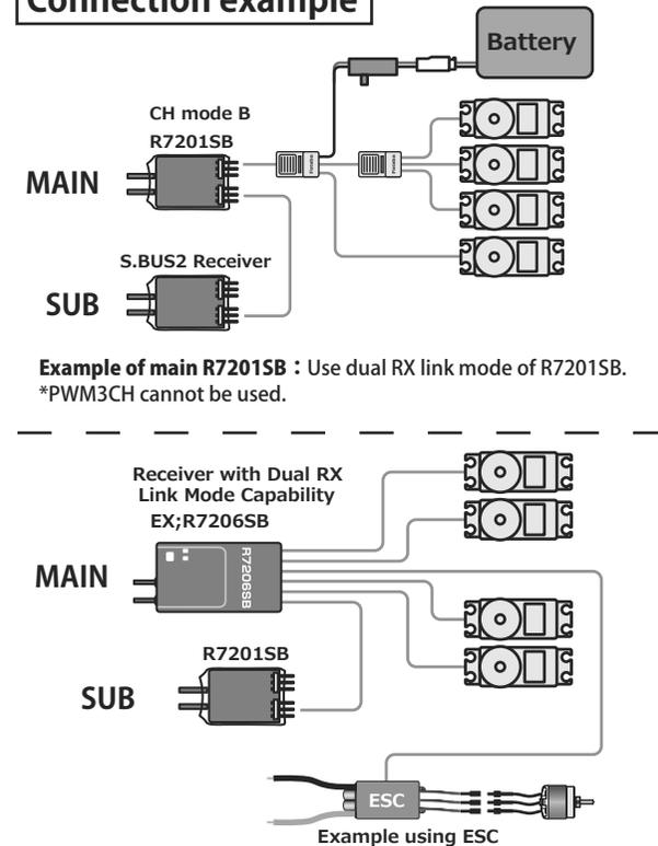
**Example of sub R7201SB :** Use dual RX link mode of R7206SB. \*Do not turn on the dual RX link mode of the R7201SB.
