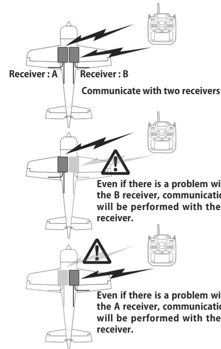
In Dual RX link mode, the S.BUS2/RX port is for reception only, so use separate ports for S.BUS output and S.BUS2 input/output.
