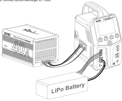
3. Discharge the battery by connecting to T1000 on Port A;
