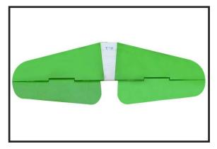
7) When you are sure that everything is aligned correctly, mix up a generous amount of 30 Minute Epoxy. Apply a thin layer to the top and bottom of the stabilizer mounting area and to the stabilizer mounting platform sides in the fuselage. Slide the stabilizer in place and realign. Double check all of your measurements once more before the epoxy cures. Hold the stabilizer in place with T-pins or masking tape and remove any excess epoxy using a paper towel and rubbing alcohol.
