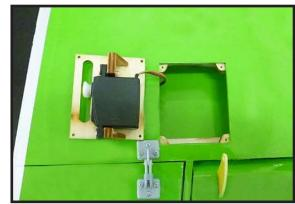
8) Set the aileron hatch in place and use a Phillips screw driver to install it with four wood screws.
