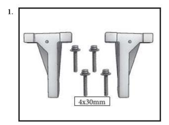
2) Use four 4x30mm head bolts and four 4mm washers to attach the engine mount rails to the fiewall. Tighten the screws . Make sure to use threadlock on the screws to help prevent them from vibrating loose.
