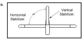
4) Slide the vertical stabilizer back inplace. Using a triangle, check to ensure that the vertical stabilizer is aligned 90° to the horizontal stabilizer.
