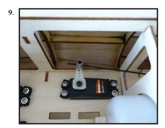
9) Move the throttle stick to the closed position and move the carburetor to closed. Use a 2.5mm hex wrench to tighten the screw that secures the throttle pushrod wire. Make sure to use threadlock on the screw so it does not vibrate loose.
