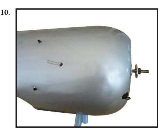
4) Install the muffler and muffler extension onto the engine and make the cutout in the cowl for muffler clearance. Connect the fuel and pressure lines to the carburetor, muffler and fuel filer valve. Secure the cowl to fuselage using the M3x10mm socket head screws. Putting a small length of silicon fuel tube under the head of the screw helps with vibration.
