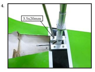
2) Install servo for Retractable landing gear.
