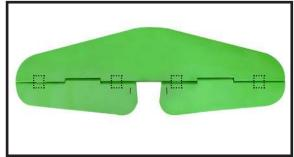
INSTALL ELEVATOR CONTROL HORN.
