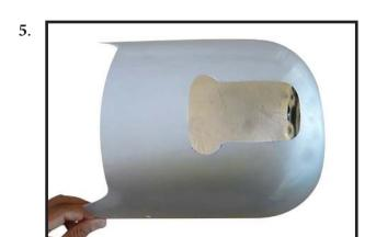
1) Tape the cowl to the fuselage using low-tack tape.
