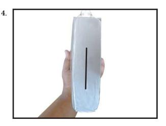
3) While holding the vertical stabilizer fimly in place, use a pen and draw a line on eachside of the vertical stabilizer where it meets the top of the fuselage.
