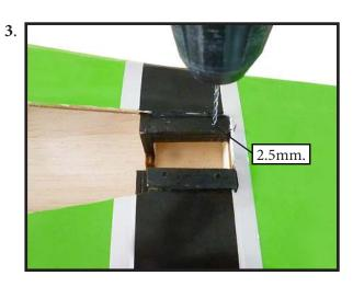
INSTALLING LANDING GEAR.
