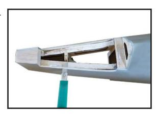
3) Slide the stabilizer into place in the precut slot in the rear of the fuselage. The stabilizer should be pushed firmly against the front of the slot.
