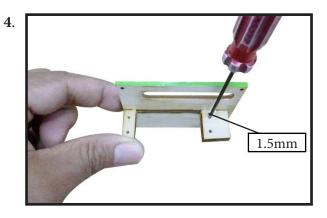
3) Apply 2-3 drops of thin C/A to each of the mounting holes. Allow the C/A to cure without using accelerator.
