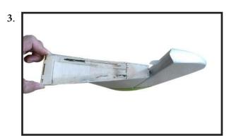
2) Slide the vertical stabilizer into the slot in the top of the fuselage. The rear edge of the stabilizer should be flsh with the rear edge of the fuselage and the lower rudder hinge should engage the precut hinge slot in the lower fuselage. The bottom edge of the stabilizer should also be fimly pushed against the top of the horizontal stabilizer.
