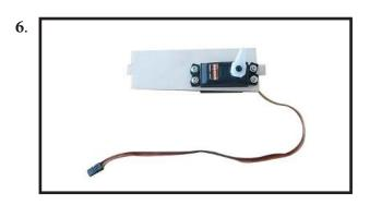
**Minimum servo spec. Torque**: 222 oz-in (16 kg-cm) @ 4.8V; 278 oz-in (20 kg-cm) @ 6.0V
