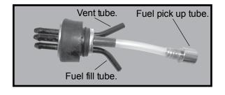
3) Carefully bend the second nylon tube up at a 45° angle. This tube is the vent tube.
