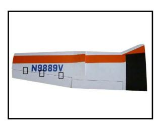
Note: Work the aileron up and down several times to "work in" the hinges and check for proper movement.
