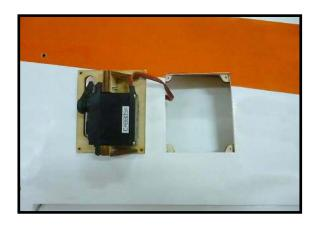
8) Set the aileron hatch in place and use a Phillips screw driver to install it with four wood screws.
