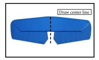
2) Using a modeling knife, carefully remove the covering at mounting slot of horizontal stabilizer ( both side of fuselage).
