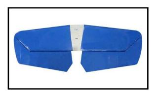
□ 7) When you are sure that everything is aligned correctly, mix up a generous amount of 30 Minute Epoxy. Apply a thin layer to the top and bottom of the stabilizer mounting area and to the stabilizer mounting platform sides in the fuselage. Slide the stabilizer in place and realign. Double check all of your measurements once more before the epoxy cures. Hold the stabilizer in place with T-pins or masking tape and remove any excess epoxy using a paper towel and rubbing alcohol.
