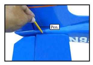
$\Box$  5) Remove the stabilizer. Using the lines you just drew as a guide, carefully remove the covering from between them using a modeling knife.
