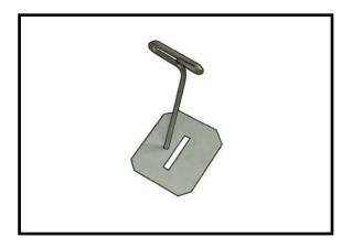
2) Remove each hinge from the wing panel and aileron and place a T-pin in the center of each hinge. Slide each hinge into the wing panel until the T-pin is snug against the wing panel. This will help ensure an equal amount of hinge is on either side of the hinge line when the aileron is mounted to the aileron.
