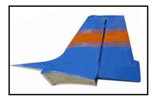
1) Using a modeling knife, remove the covering from over the precut hinge slot cut into the lower rear portion of the fuselage. This slot accepts the lower rudder hinge.
