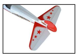
5) When you are sure that everything is aligned correctly, mix up a generous amount of Flash 30 Minute Epoxy. Apply epoxy to the bottom and top edges of the filler block. Set the stabilizer in place and realign. Double check all of your measurements once more before the epoxy cures. Hold the stabilizer in place with T-pins or masking tape and remove any excess epoxy using a paper towel and rubbing alcohol. Allow the epoxy to fully cure before proceeding.
