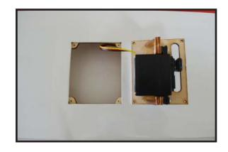
8) Set the aileron hatch in place and use a Phillips screw driver to install it with four wood screws.
