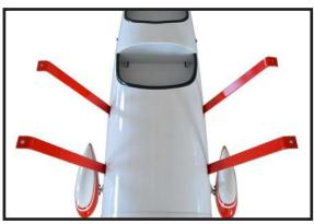
3) Place the upper center wing rib in position on the cabane struts. Start the M3 x 12 socket head machine screws and M3 washers that secure the rib to the cabane struts.
