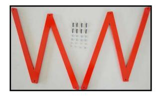
2) Attach the two wing struts to the top of lower wing pant using an M3x12mm nachine screw and M3 washers.
