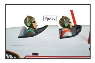
4) Position the windshield onto the fuselage. Trace around the windshield onto the fuselage using a felt-tipped pen. Cut and remove the covering from between the lines drawn, and glue the windshield to the fuselage using epoxy or a special canopy glue.
