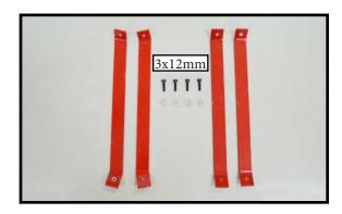
2) Place the cabane struts in position, noting their position as shown in the photo. Loosely install the four M3 x 12 socket head machine screws and M3 washers. Leave the hardware loose so the struts can be positioned while installing the upper wing center rib. Make sure to use threadlock on the screws so they won't vibrate loose.
