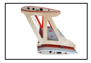
Using the transport frames allow the removal of the wings without the need to remove the aileron linkage and the interplane strut between the top and bottom wings.
