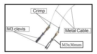
2) Attach the clevis to the brass tab next to the rear interplane strut on the upper-lower wing. Slide a copper crimp on the cable. Pass the cable through the brass tab on the upper wing, the back through the copper crimp.
