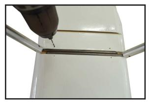
Thread a mounting screw into each of the holes to cut threads in the surrounding wood. Apply a small amount of thin CA to harden the threads make by the screws. Position the landing gear so it rakes forward. Use the screws and landing gear straps to secure the landing gear to the bottom of the fuselage.
