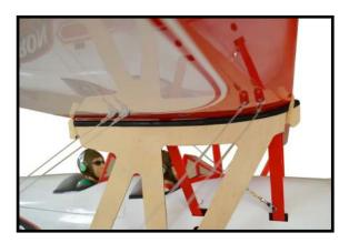
2) Use a 2.5mm hex wrench to remove the screws that attach the panels to the fuse-lage and center section. Slide the panels from the tubes and disconnect the servo lead for the aileron servo.
