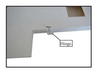
3) Slide the wing panel on the aileron until there is only a slight gap. The hinge is now centered on the wing panel and aileron. Remove the T-pins and snug the aileron against the wing panel. A gap of 1/64" or less should be maintained between the wing panel and aileron.
