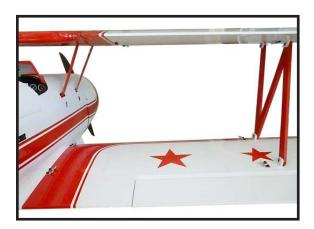
At this time, exact position of the end is set, please Use a 2.5mm hex wrench to slowly tighten the hardware securing the cabane struts in position on the fuselage. Again, make sure to use threadlock on all the fasteners to prevent them from vibrating loose.
