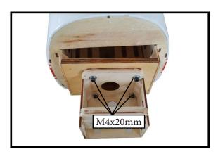
4) Attach the motor to the front of the electric motor box using four 4mm blind nut, four M4x20mm hex head bolts to secure the motor. Please see picture shown.
