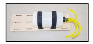
You should mark which tube is the vent and which is the fuel pickup when you attach fuel tubing to the tubes in the stopper. Once the tank is installed inside the fuselage, it may be difficult to determine which is which.
