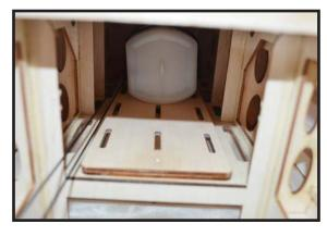
8) Use balsa block to hold in place the fuel tank with C/A glue to secure the fuel tank inside the fuselage.
