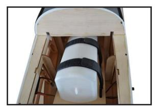
7) Slide the fuel tank into the fuselage. Guide the lines from the tank through the hole in the firewall.
