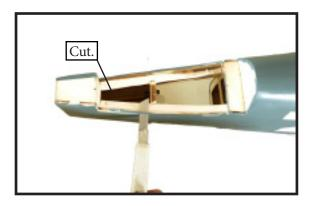
3) Slide the stabilizer into place in the precut slot in the rear of the fuselage. The stabilizer should be pushed firmly against the front of the slot.
