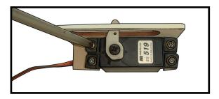
7) Apply 1-2 drops of thin C/A to each of the mounting tabs. Allow the C/A to cure without using accelerator.
