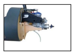
8) Reinstall the servo horn by sliding the connector over the pushrod wire. Center the throttle stick and trim and install the servo horn perpendiular to the servo center line.
