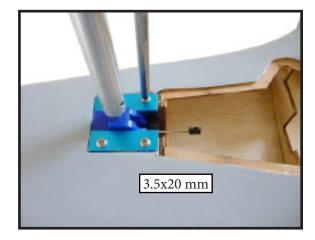
2) Install servo for Retractable landing gear.
