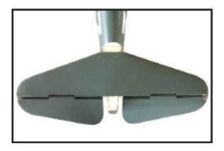
4) With the stabilizer held firmly in place, use a pen and draw lines onto the stabilizer where it and the fuselage sides meet. Do this on both the right and left sides and top and bottom of the stabilizer.
