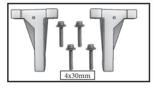
2) Use four 4x30mm head bolts and four 4mm washers to attach the engine mount rails to the firewall. Tighten the screws . Make sure to use threadlock on the screws to help prevent them from vibrating loose.
