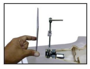
Secure the landing gear doors to the landing gear struts.
