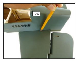
5) Remove the stabilizer. Using the lines you just drew as a guide, carefully remove the covering from between them using a modeling knife.
