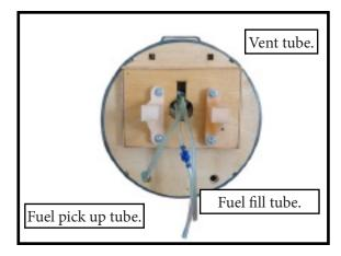
8) Connect the lines from the tank to the engine and muffler. The vent line will connect to the muffler and the line from the clunk to the carburetor.
