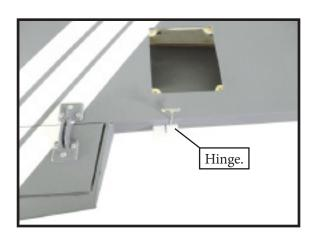
3) Slide the wing panel on the aileron until there is only a slight gap. The hinge is now centered on the wing panel and aileron. Remove the T-pins and snug the aileron against the wing panel. A gap of 1/64" or less should be maintained between the wing panel and aileron.
