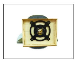
4) Attach the motor to the front of the electric motor box using four 4mm blind nut, four M4x20mm hex head bolts to secure the motor. Please see picture shown.
