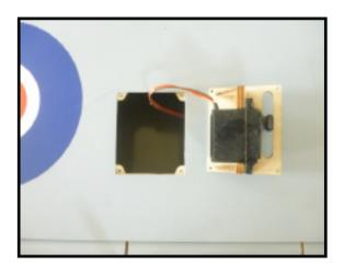
9) Set the aileron hatch in place and use a Phillips screw driver to install it with four wood screws.
