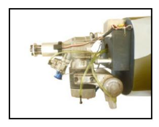
1) Reinstall the servo horn by sliding the connector over the pushrod wire. Center the throttle stick and trim and install the servo horn perpendicular to the servo center line.
