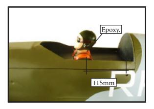
4) Position the canopy onto the fuselage. Trace around the canopy and onto the fu¬selage using a felt-tipped pen. Carefully cut and remove covering material from the fusealge where the canopy makes contact, exposing the bare wood. The permanently glue the canopy in place with epoxy glue or special "canopy glue".
