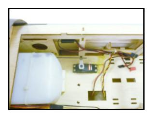
2) Move the throttle stick to the closed position and move the carburetor to closed. Use a 2.5mm hex wrench to tighten the screw that secures the throttle pushrod wire. Make sure to use threadlock on the screw so it does not vibrate loose.
