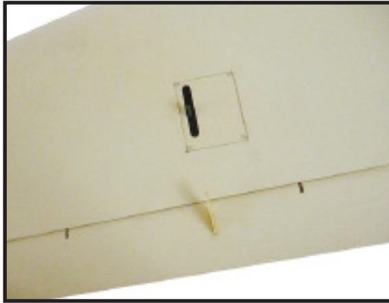
INSTALLING THE FLAP SERVOS.
