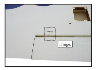
4) Deflect the aileron and completely saturate each hinge with thin C/A glue. The ailerons front surface should lightly contact the wing during this procedure. Ideally, when the hinges are glued in place, a 1/64" gap or less will be maintained throughout the lengh of the aileron to the wing panel hinge line.
