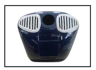
2) While keeping the back edge of the cowl flush with the marks, align the front of the cowl with the crankshaft of the engine. The front of the cowl should be positioned so the crankshaft is in nearly the middle of the cowl opening. Use the spinner backplate as a guide. Hold the cowl firmly in place using pieces of masking tape.
