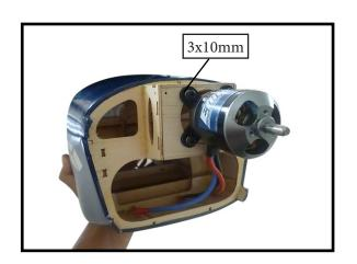
2) Connect the leads from the motor to the speed control. Use hook and loop tape to mount the speed control in the fuselage. Make sure to the position the speed control far enough into the fuselage so the lead from the speed control can be connected to the receiver. Use tiewraps to secure the wiring so it doesn't interfere with the operation of the motor.
