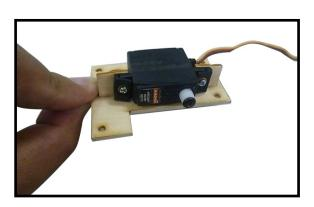
7) Apply 1-2 drops of thin C/A to each of the mounting tabs. Allow the C/A to cure without using accelerator.
