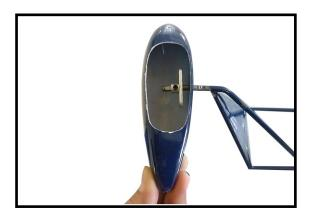
Slide the wheel pant and wheel onthe landing gear. With both wheels and pants place, rest the fuselage on the flat surface. Check that there is clearance between the surface and wheel pant. Tighten the setscrews so they leave marks on the axle.
