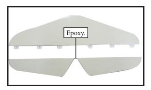
Glue the hinge hinges in place using the same techniques used to hing the ailerons.
