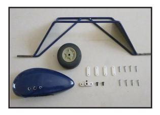
Thread a mounting screw into each of the holes to cut threads in the surrounding wood. Apply a small amount of thin CA to harden the threads make by the screws. Position the landing gear so it rakes forward. Use the screws and landing gear straps to secure the landing gear to the bottom of the fuselage.
