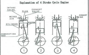
The four-stroke engine consists of four individual piston movements as illustrated above.
