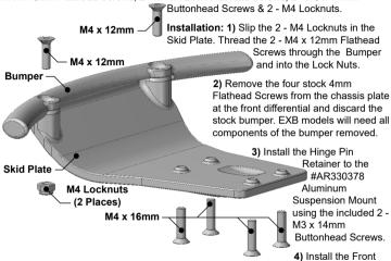
Bumper assembly on the chassis using the included 4 - M4 x 16mm Flathead Screws.
