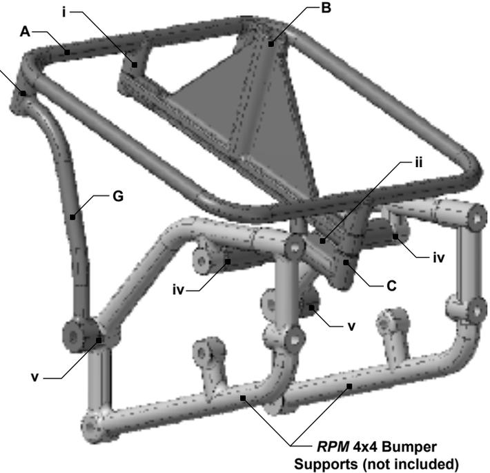
Letters  (A) Support Loop, (B) Tire Mount, (C) 4x4 Rear Brace, (D) 2wd Rear Brace, (E) 2wd Shock Tower Adapter, (F) 2wd Front Braces & (G) 4x4 Front Braces.
