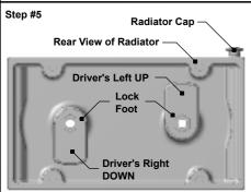
Orient the **Lock Feet** as shown here. Failure to orient the **Lock Feet** correctly will make it difficult to attach the body of the truck to the **Lock Plate** after bolting the **Radiator** to the body.
