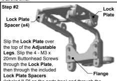
(labeled "LP" on the parts tree) and through the Adjustable Legs. Secure in place using 4 - M3 Locknuts. Bolt the Rear Shock Tower Bracket to the shock tower using stock screws. The flange of the Rear Shock Tower
