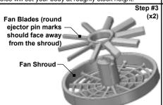
Slip the Fan Blade over the post of the Fan Shroud, making sure the ejector pin marks on the Fan Blade face away from the Fan Shroud. Repeat for both Fan Blades / Fan Shrouds.
