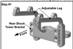
Bolt the **Adjustable Legs** to the **Shock Tower Bracket** using 4 - M3 x 10mm Flathead Screws. Counting from the top of the **Adjustable Legs**, the second and fourth holes will set your body at roughly stock height.
