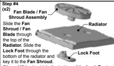
Slip an M3 Locknut into the bottom of the **Lock Foot**. Slip 1 - M3 x 25mm Buttonhead Screw through the top of the **Fan Shroud** and tighten with the locknut in the **Lock Foot**. The **Fan Shroud** should be able to rotate freely. Repeat for both **Fan Shrouds** / **Fan Blades**.
