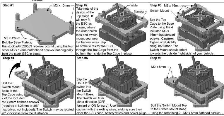
The RPM ESC Cage is very versatile and can be mounted practically anywhere given enough space to drill & tap four 3mm mounting holes and fit the base plate.
