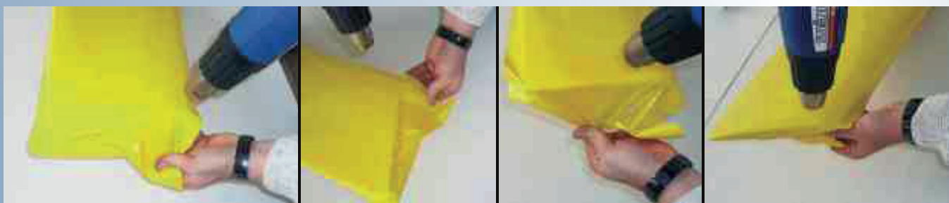
Fig. 11a-d Covering of the wing tip
