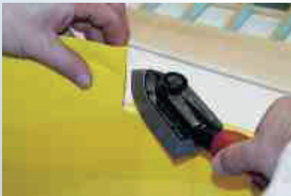
Fig. 12b Fold and bond covering.
