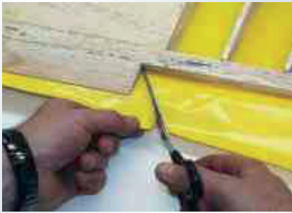
Fig. 12a For Inside corners, first slit 45°.
