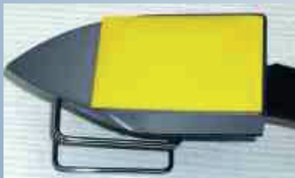
Fig. 3A Temperature test at approx. 90°C
