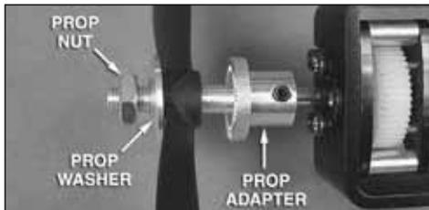
Slide the prop adapter over the output shaft of the gear drive or motor. Align one of the set screws with the flat on the output shaft of the gear drive. Apply a drop of Great Planes **Threadlocker (GPMR6060)** to the set screw and install it in the prop adapter, tightening it against the flat of the gear drive output shaft. Remove the second set screw that does not tighten onto the flat. When installing the prop
