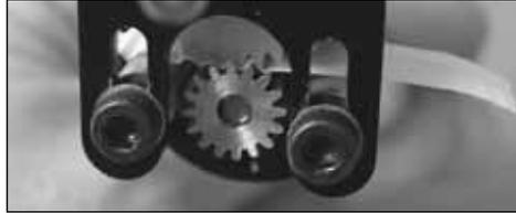
Loosely mount the motor to the back of the back plate with two 3x20mm SHC screws and two 3mm flat washers. Place a piece of notebook paper between the pinion gear and the spur gear. Squeeze the two gears together while tightening the two 3x20mm SHC screws. Remove the piece of paper and the gear mesh should be set. Rotate the gears to make sure they rotate smoothly. If they do not, slightly loosen the gear mesh until the gears do rotate smoothly.
