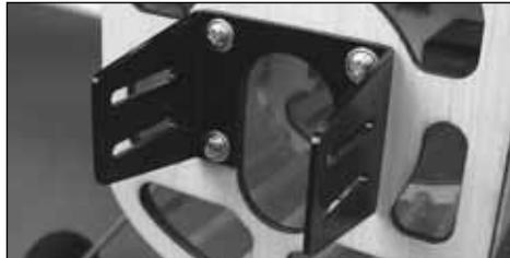
Attach the Backplate to the firewall using four 4-40 machine screws and four #4 flat washers. Note that if you are using a gear drive you may have to cut a hole in the firewall for the motor. Most motors and gear drives can be mounted to the Front Plate using 3mm machine screws. If you are using a different gear drive other than the Great Planes gear drive, the hole locations may need to be modified.
