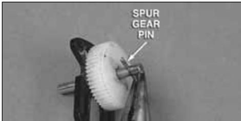
Press the output shaft out of the spur gear and remove the spur gear pin. The spur gear can now be replaced. Reverse the order to reassemble the gear drive. Be sure to use a drop of threadlocker on the two 2.5x17mm flat head machine screws to prevent them from loosening during operation.
