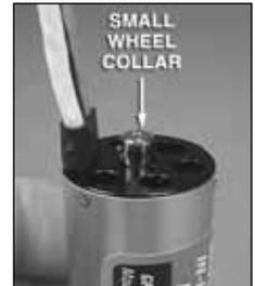
for supporting the motor shaft. If you have a drill press the motor can be placed in a vise with the motor shaft supported on a small wheel collar. Use a small micro torch to heat the pinion gear and use the drill chuck of the drill press to press the pinion onto the shaft.
