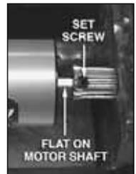
Once the pinion gear is in position on the motor shaft, apply a drop of threadlocker to the threads of the set screw and tighten it down on the flat of the motor shaft.
