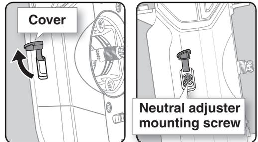
**2** Move the adjuster lever up and down to determine the neutral position.
