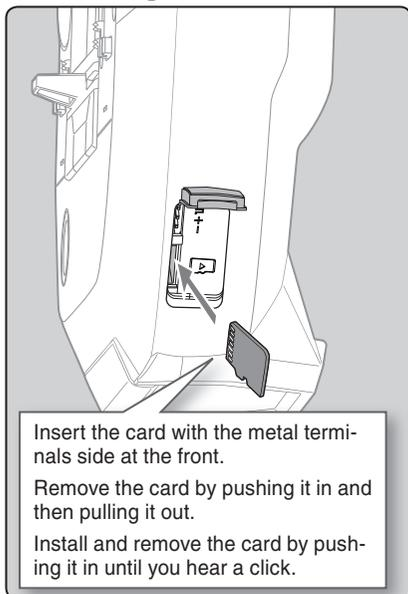
Insert the card with the metal terminals side at the front.
