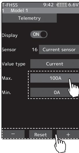
Tap the value button of the [Max.] and [Min]. Value input buttons appear on the screen. Use the [+] and [-] buttons to adjust the upper limit and lower limit amount.
