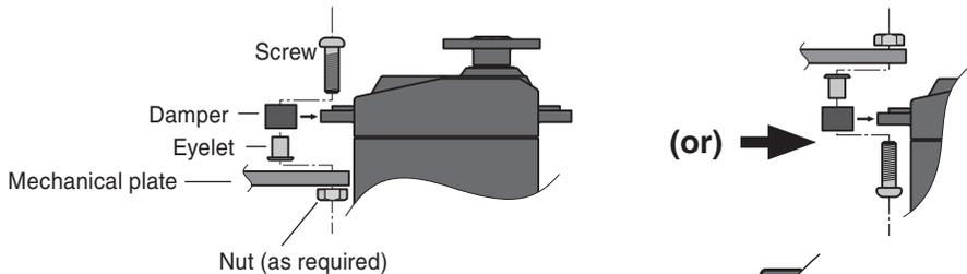
When installing the servo, always install the accessory rubber grommet and grommet flush against the servo.
