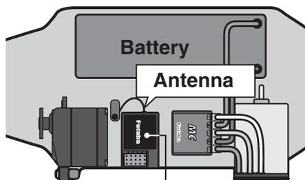
Install the receiver as far away as possible from the battery, motor controller, motor, silicon cord and other noise sources. Keep it away from the antenna wire, in particular.
