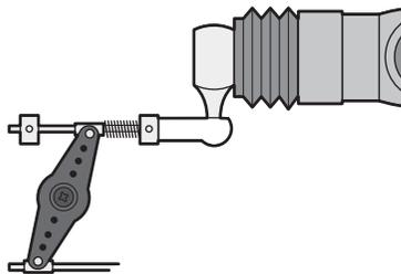
Adjust the throttle servo so that unreasonable force is not applied when the engine carburetor is fully open, fully closed, and the brakes are applied fully. If the brakes overheat while running, their ability to function properly decreases. Before running, adjust the suitable maximum servo travel so that unreasonable force is not applied even when the servo travel is increased while running.
