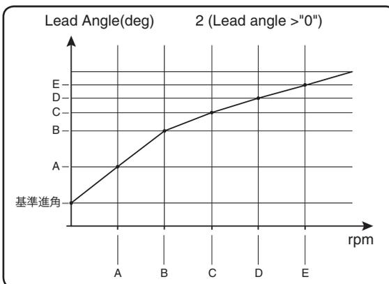
When using in races in which the lead angle setting function is inhibited by the ESC, set "Lead angle use" to "INH". The "Lead angle use" setting has priority over "Turbo mode". If "Lead angle use" is set to "INH", the lead angle setting function can be turned off even if "Turbo mode" is set to "Turbo 1" or "Turbo 2".
