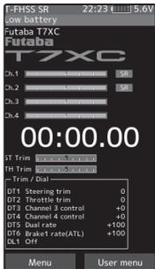
If the transmitter battery voltage drops below the usable range, an audible alarm will sound and "Low battery" will be displayed. Since the usable range of LiFe and NiMH batteries are different, the power supply used must be set by system setting (page 180).
