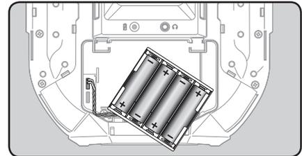
**3** Insert the connector of the new battery and load the new battery into the transmitter.
