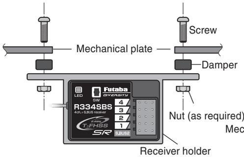
When using the receiver holder supplied with the kit, install the receiver through a rubber grommet.
