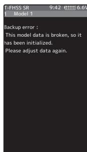
If the data in the transmitter is not transferred normally when the power is turned on, an audible alarm will sound and "Backup error" will be displayed on the LCD.
