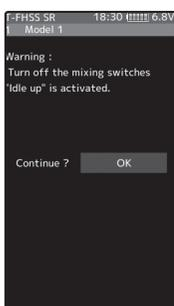
If "Throttle mode" is changed to "Forward 100 : Brake 0", the throttle stick is not in the stop/idle position when the power switch is turned on, an audible alarm will sound and "Warning" will be displayed on the LCD. When the throttle stick is thrown will stop.
