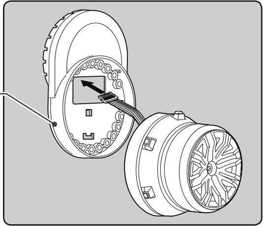
**5** Using a Phillips screwdriver fasten the wheel unit and APA at the desired angle using the 2.6x19mm tapping screws. Be careful that the screw length is correct. Be careful that the wiring does not get pinched. The angle can be adjusted, but check the marking point on the wheel unit and install the screws.
