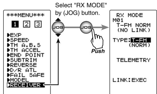
**2** Move the cursor to "TYPE: ----" by the (JOG) button up or down operation, and select the RX type with the (+) button or (-) button.
