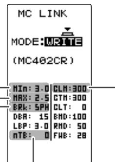
"Min", which sets the frequency when the load is small, is set to the high frequency side (large value) when extension is desired after straightaways and curves.
