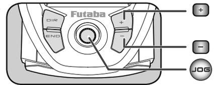
**1** Call the MENU 1 screen from the HOME screen by moving the (JOG) button up, down, left or right. Select "RECEIVER" by moving the (JOG) button up or down, and display the "RX MODE" screen by pressing the (JOG) button.
