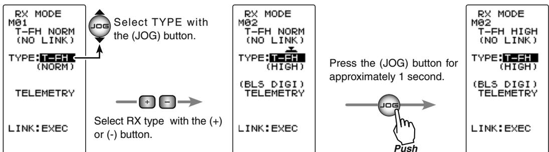
\*When using an S-FHSS(SFH) system (R2104GF, R204GF-E, etc.) receiver, after reaching this point set the transmitter power switch to OFF and go to "Receivers other than T-FHSS" on page 36.
