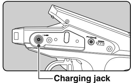
Charge the optional FT2F1700B/2100B (LiFe) battery with the special charger in accordance with the instruction manual supplied.
