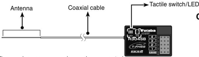
The receiver power supply can be connected to the S.BUS2 connector or each of CH1-4.
