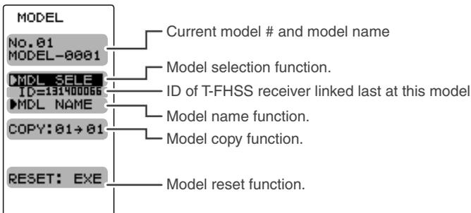
When a T-FHSS receiver is not linked with a model whose RX type is set to T-FHSS, (NO LINK) is displayed.
