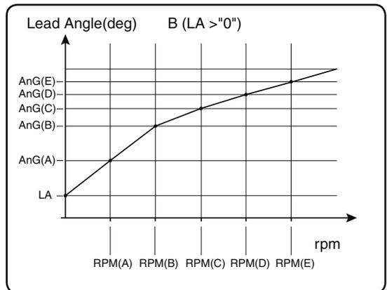
When using in races in which the lead angle setting function is inhibited by the ESC, set LAU (LEAD ANGLE USE) to OFF. The LAU setting has priority over TBM-(TURBO MODE). If LAU is set to "OFF", the lead angle setting function can be turned off even if TBM is set to "LV1" or "LV2". The MC940,960CR shows that the lead angle setting function is OFF ("0" timing) by blinking a LED.
