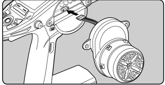
**8** Install the assembled steering wheel unit and APA to the transmitter using the screw (3.0x12mm cap screw) supplied.
