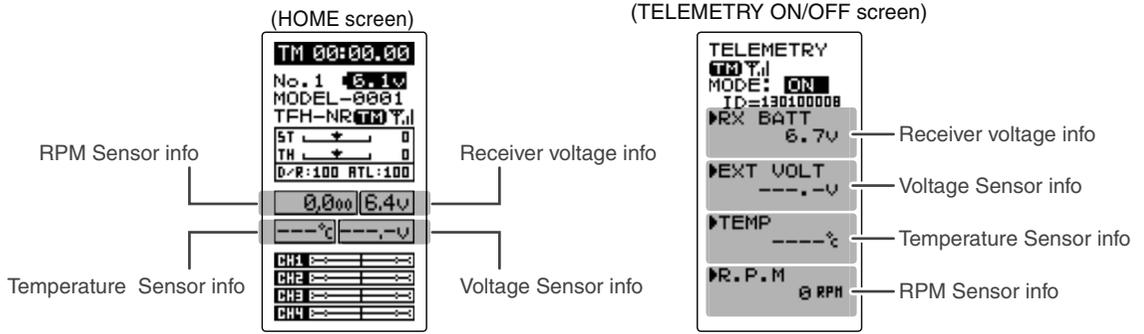
Display "TELEMETRY" screen using the following method:
