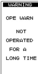
If the T4PV is not operated for 10 minutes, an audible alarm is sounded and "OPE WARN" is displayed on the screen. The audible alarm stops when the steering wheel, throttle trigger, and any dial, switch, or edit button is operated. If you are not going to use the transmitter, turn the power off. (Setting can be reset at the system menu on page 123.)
