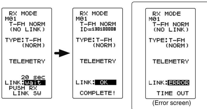
\*The T4PV and a telemetry type T-FHSS receiver (R304SB, etc.) mutually memorize the combined ID linked last at each model memory.
