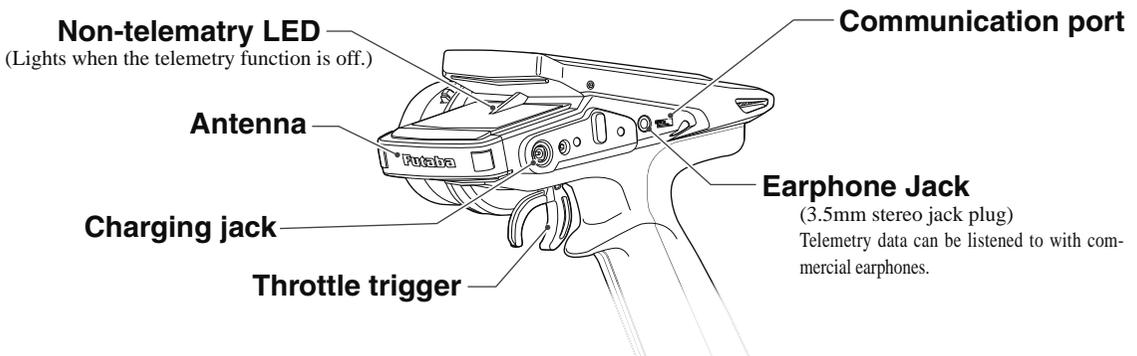
\*The switches, dial, and trimmers in the figure are shown in the initial setting position.
