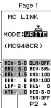
"Min", which sets the frequency when the load is small, is set to the high frequency side (large value) when extension is desired after straightaways and curves.
