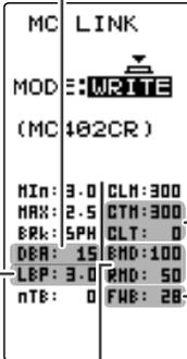
**CTM-(C.L. TIME LIMIT) 50A~300A /CLT-(C.L. TIMER) 0sec(OFF)~240sec (except MC950CR)**
