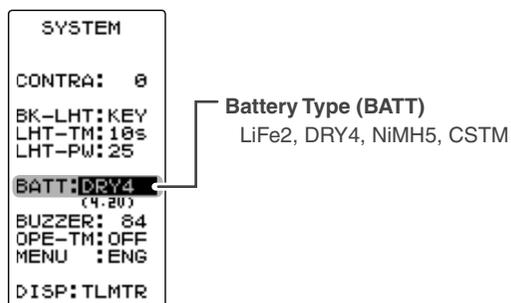
When finished with setting, return to the MENU screen by pressing the (END) button.
