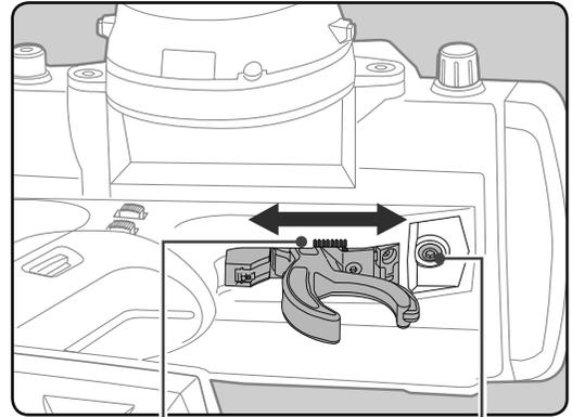
Trigger slide mounting screw
