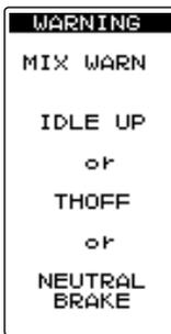
When the power switch is turned on while the idle-up, preset (engine cut) or neutral brake function switch is on, an audible alarm will sound and "MIX WARN" will be displayed on the LCD. When that function switch is turned off, the alarm will stop.
