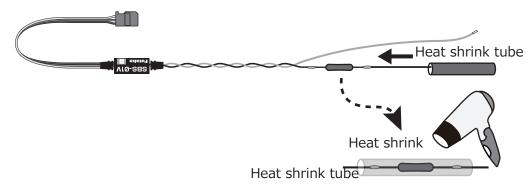
4 The cable should be connected as shown in the diagram below. The cable gets connected to the wires that come off the ESC and connect to the battery.
