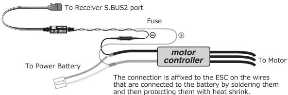
**⑤** The manual for the Telemetry system should be referred to after the setup is complete; checking to make sure it functions as desired and that it provides the correct voltage on the display.
