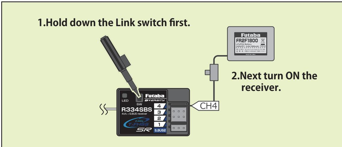
5. Once LED confirms by the "red flashing once", release the Link switch, and re press again.
