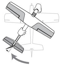
Tilt the airplane to the left on the ground and check that the ailerons operate to the right. Tilt the airplane to the up on the ground and check that the elevator operate to the down.
