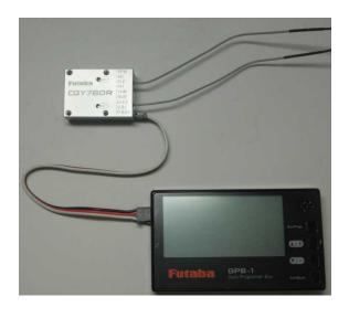
Connection of GPB-1 and Transmitter
