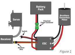
2028 motors only. DO NOT CUT any part of the wire length from any other motor, regardless of brand or type. In most cases, only the last 1/4 inch or so of the motor wires are able to be soldered. If they are clipped shorter you may not be able to solder the remaining portion of the wire and the motor will not run properly, if at all.
