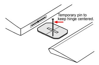
2) Apply drops of thin CA to the top and bottom of each hinge. Do not use CA accelerator. After the CA has fully hardened, test the hinges by pulling on the aileron.
