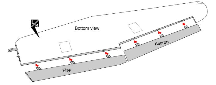
1) Test fit the ailerons to the wing with the hinges. If the hinges don't remain centered, stick a pin through the middle of the hinge to hold it in position.
