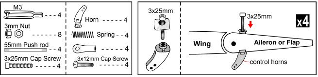
Remove the covering from the slot on the bottom of the aileron. Insert the control horn into the slot and secure.
