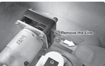
1. Remove the water line between the water pick up tube and water pump.
