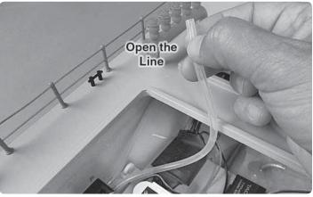
3. Install the open end of the line back onto the pump. Then, soften your grip on the pinched end of the line. The water in the line will go into the pump to provide the prime.
