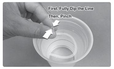
2. Fully submerge the line in water. Pinch the end closed as vou remove the line from the water.
