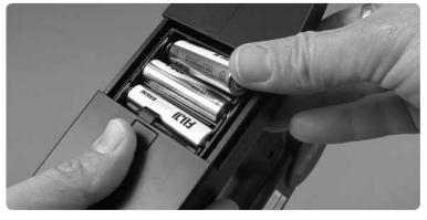
Install 4 AA batteries into the transmitter using the installation pattern molded into the bottom of the battery tray.
