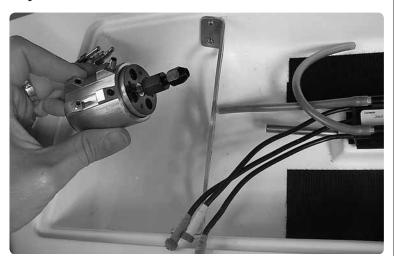
Remove the motor from the boat.
