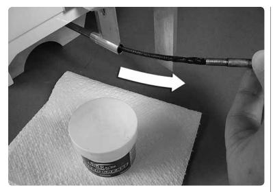
Firmly pull the prop and drive shaft out of the back of the boat. NOTE: If you find the shaft hard to remove try rotating the shaft clockwise as you pull.
