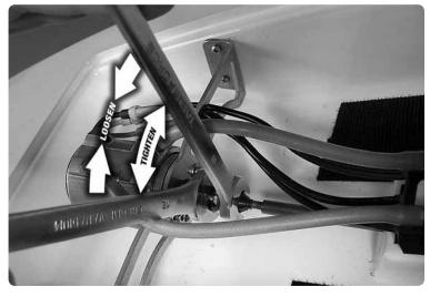
Loosen the cable coupler using the 10mm and 12mm wrenches.
