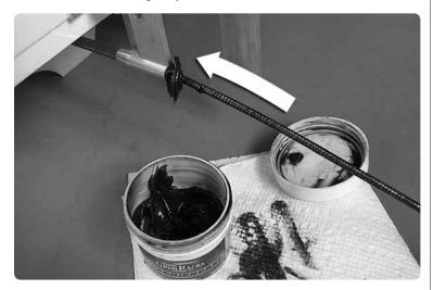
Wipe away any old grease and water. Apply new grease (AQUB9500 Speed Grease) to the shaft and slide it back into the strut, moving it in and out as you do so to help spread the grease along the length of the cable.
