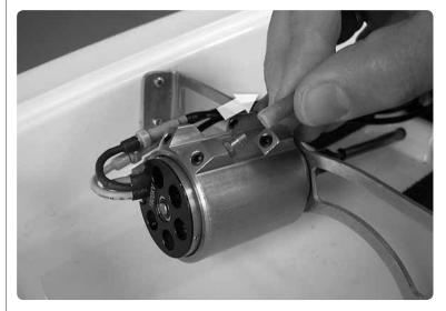
Start by removing the water lines to the motor jacket.
