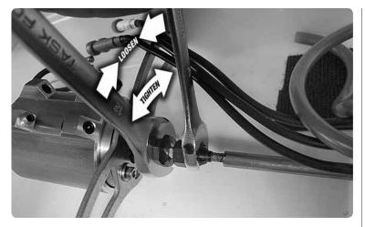
Use the 12mm and 10mm wrenches to loosen the cable coupler from the cable. To do so, hold the 12mm wrench still and rotate the 10mm wrench counterclockwise.
