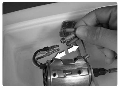
Unplug the three 4mm connector leads to the motor.
