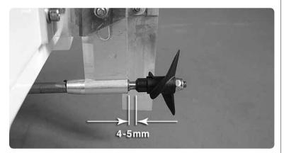
Before tightening the cable coupler, make sure to leave 4 or 5mm distance between the back of the strut and the front of the drive dog. This will keep the drive system from binding or breaking as the cable retracts during operation. Tighten the cable coupler, reversing the direction of the open end wrenches. **DO NOT OVER TIGHTEN**.
