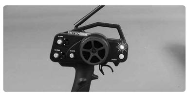
Turn on the transmitter, making sure it's working by viewing the LED on the front. The LED should glow bright red.
