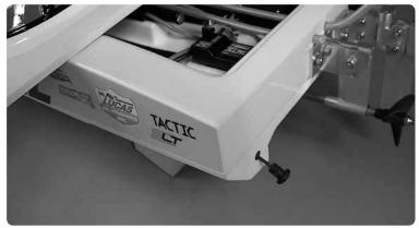
At the end of the day, make sure to leave the cowl off and the drain plug out over night. This will allow any moisture that collected in the boat to evaporate.
