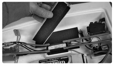
Remove the canopy and install the provided hook and loop material to your battery packs. Install the batteries, making sure they are well seated.
