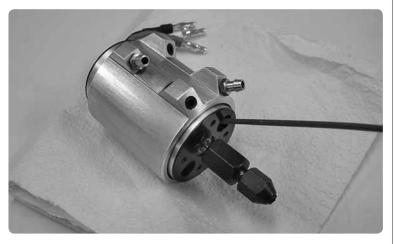
Place the motor in a rag or paper towel and spray water displacer into the fittings on the water jacket as well as in the motor itself.
