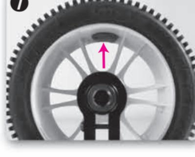
It may be necessary to repeat the procedure a few times to verify the wheel balance. Repeat the procedure until the wheel stops in a different position each time.
