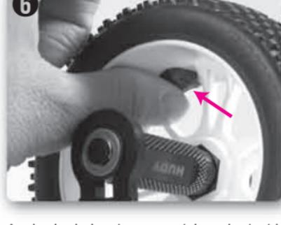
Apply the balancing material to the inside of the wheel, OPPOSITE to the heavy side at the bottom of the wheel. The balancing material must be pressed to the edge of the wheel so it stay firmly in place when you run the car. The quantity of the balancing material depends on how unbalanced the wheel is.
