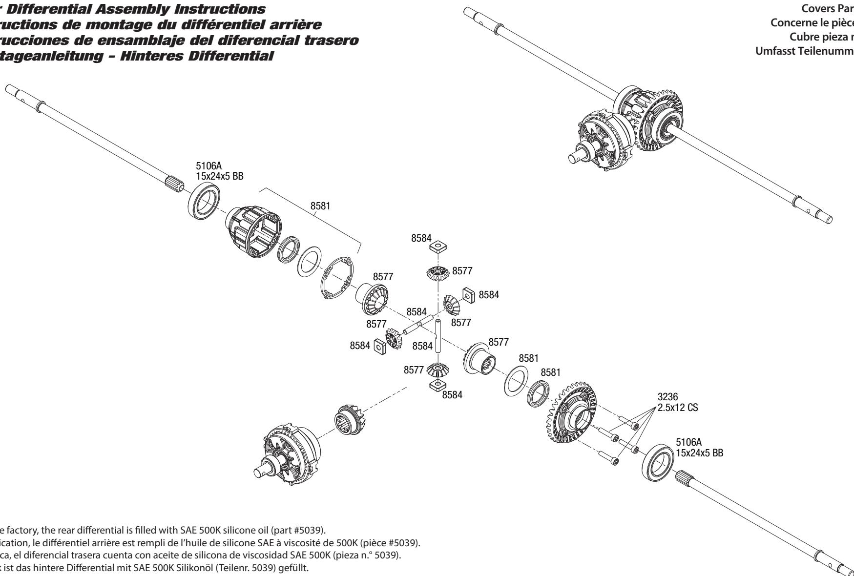
From the factory, the rear differential is filled with SAE 500K silicone oil (part #5039).
