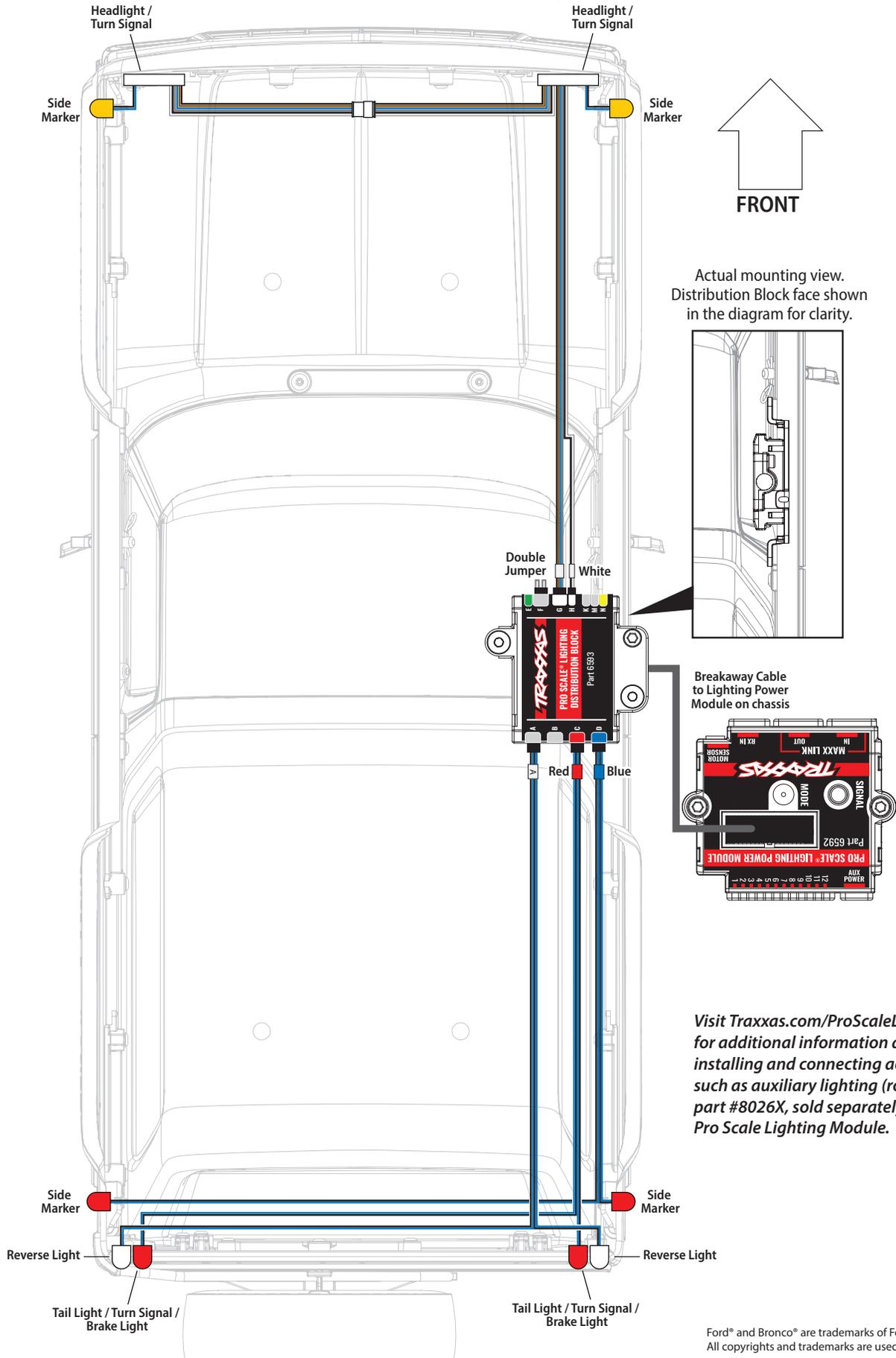
Visit [Traxxas.com/ProScaleLighting](http://Traxxas.com/ProScaleLighting) for additional information about installing and connecting accessories such as auxiliary lighting (rock lights, part #8026X, sold separately) to the Pro Scale Lighting Module.
