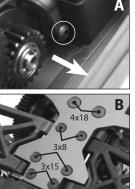
15. Remove the two-speed hub/gear assembly from the right half. (M) **Note:** The two-speed hub/gear assembly is not used with the single-speed conversion.
