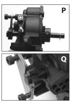
20. Move the single-speed shaft to allow room for the brake disc. Place the brake disc between the two brake pads and insert the shaft/brake disc hub assembly into the
