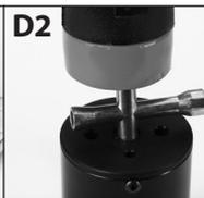
2. Drop one of the included bearings down into the motor can. Position it over the recessed bearing boss inside the can. Position an over-sized Phillips screwdriver tip into the center of the bearing and work it around until the bearing is settled evenly into the motor can (E). Use a mallet to tap the bearing the rest of the way into the can.
