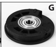
3. Place the end bell (outside down) on a wood block. Place the new 6x17x6mm bearing in the end bell housing. Place another wood block on top of the bearing and tap the bearing into the end bell with a plastic mallet (F). Make sure the bearing is fully seated (G).
